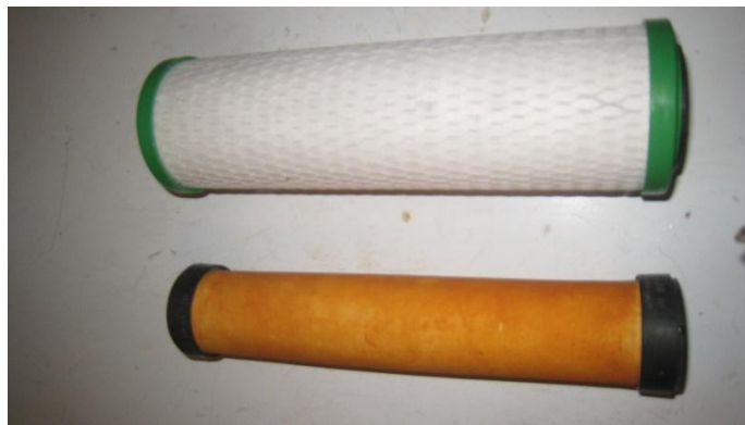
Photo 6: Stage 1 filter (lower), before cleaning. Upper photo is of the Stage 2 Lead (chemical) filter. The brown scum on the Stage 1 filter accumulates within the first few hours of use, still, in July 2016.
